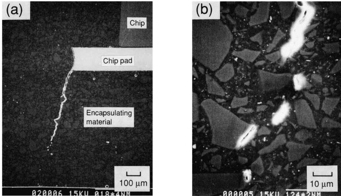
**Figure 4** Polished-appearing surfaces for cross sections of IC packages during the TST observed by SEM sealed with epoxy molding compounds filled with irregular-shaped silica particles with a particle content of 70 wt %. Mean particle size of the filled silica: (a, b) 16 μm; (c) 5 μm. Dipping cycles until observation: (a, b) 30; (c) 10.
