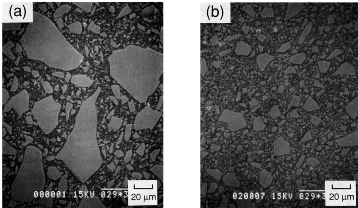
**Figure 2** SEM photographs of polished surfaces of cured epoxy molding compounds filled with irregular-shaped silica particles at a particle content of 70 wt %. Mean particle size of the filled silica: (a)  $16 \mu\text{m}$ ; (b)  $5 \mu\text{m}$ .
