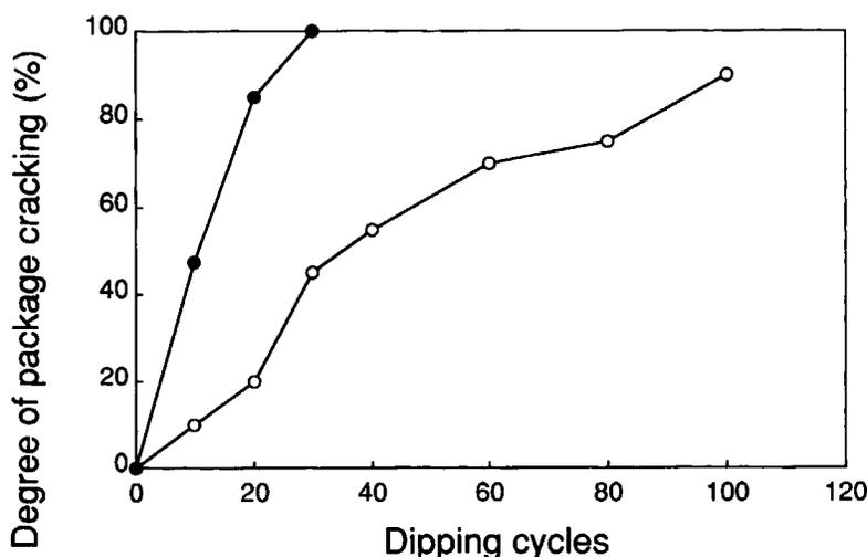
**Figure 3** Package cracks caused during the TST of IC packages sealed with epoxy molding compounds filled with irregular-shaped silica particles with a particle content of 70 wt %. Mean particle size of the filled silica: ( $\circ$ ) 16  $\mu\text{m}$ ; ( $\bullet$ ) 5  $\mu\text{m}$ .
