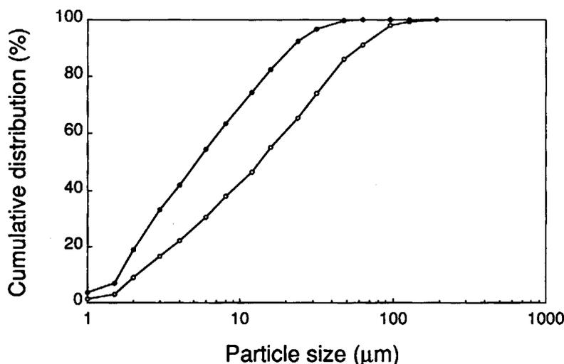
**Figure 1** Cumulative size-distribution curves for irregular-shaped silica particles. Mean particle size: (○) 16  $\mu\text{m}$ ; (●) 5  $\mu\text{m}$ .
